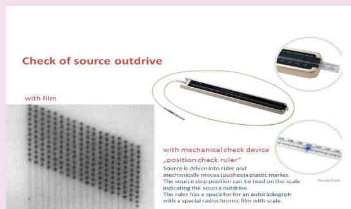
Figure 1. Example for the check of source outdrive with a source position check ruler and check of multiple channels by exposure of film with a geometric pattern of source positions (left insert).
