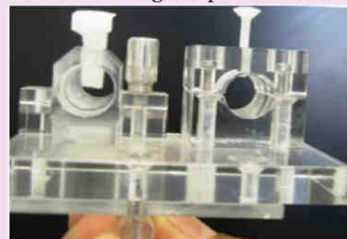
Figure-2: In-house prepared chamber mounting
