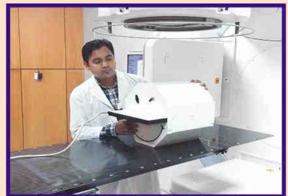
Figure-2: Plan QA using IMRT QA phantom & 2D array
