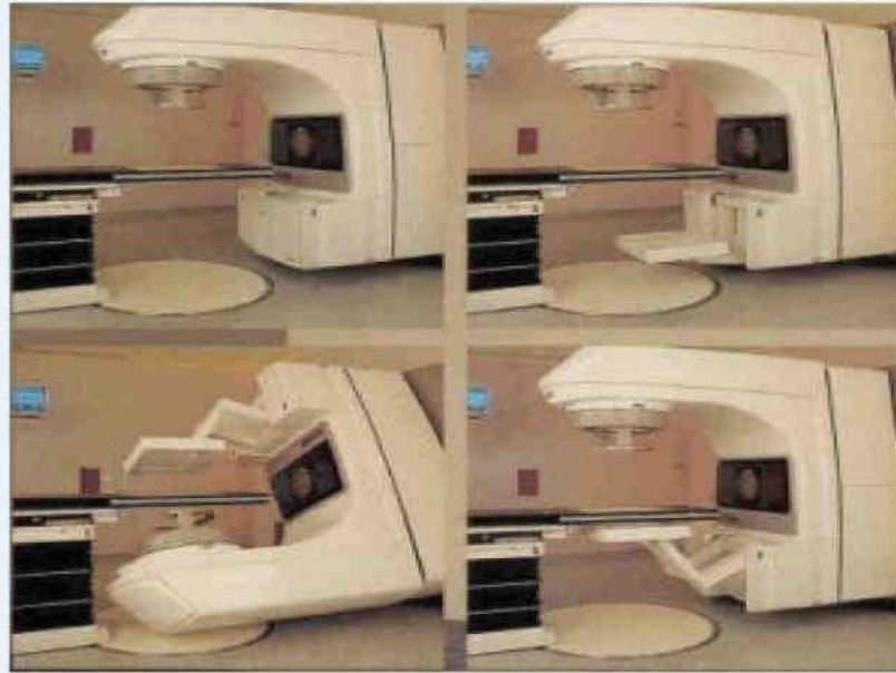
Figure 2: The new generation of EPID system is amorphous silicon based system.
