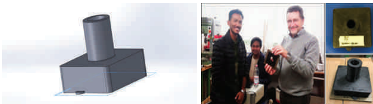
Photo: Designed and printed End term applicator using 3D printer
